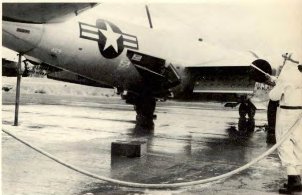
DECONTAMINATION. The most effective means of decontamination is the use of soapy water. Solvent is used to cut through grease and oil deposits.
