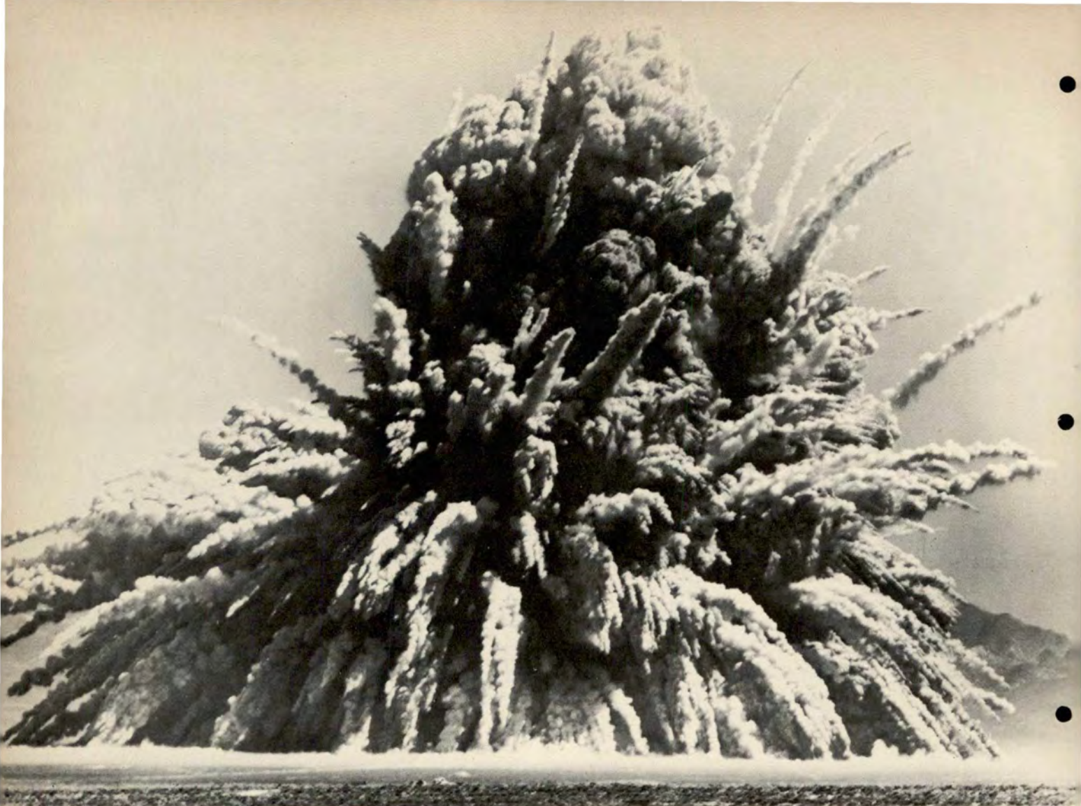
A typical nuclear excavation test at the Nevada Test Site.
