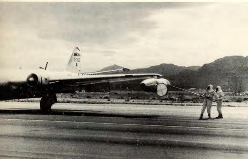
SAMPLE RECOVERY. Two members of the Sample Recovery Team pull the sample "flimsy" from the wing-tip sampling tank. Note the use of long-handled tools to keep the individual at a distance from the radioactive source.
