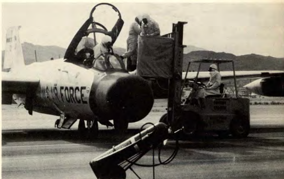
CREW RECOVERY. The crew of an RB-57C is shown climbing into a forklift-mounted box. Care is taken not to touch the contaminated aircraft exterior.
